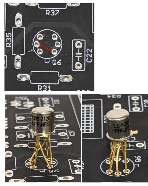
You need to keep the leads from shorting. You may want to put some insulation (like the insulation stripped from a piece of hookup wire) on one or two leads.
