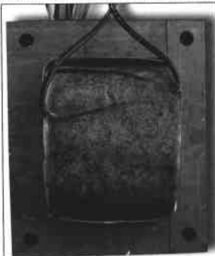
PHOTO 4: A typical EI-core transformer with the case removed.
