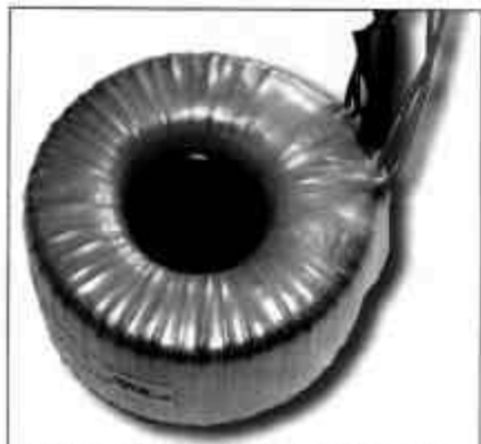
PHOTO 6: A small toroidal transformer for a tube headphone amplifier.
