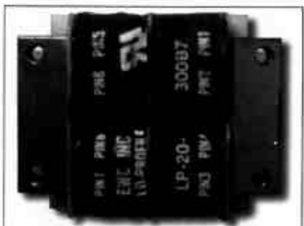
PHOTO 7: A small PCB-mount "semi-toroidal" UI-core transformer.
