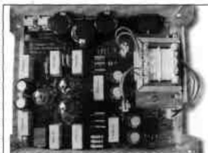
PHOTO 10: The headphone amplifier, with the EI-core transformer mounted horizontally on a bracket. Output noise due to flux leakage of this configuration was -58dBm.
