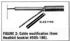
a shielded cable with two conductors inside. At one end (usually the output of the cable) the shield is connected together with one of the conductors to ground, and at the other end the shield is left unconnected. This prevents the flow of current through the shield, which can sometimes introduce noise into the signal inside.
