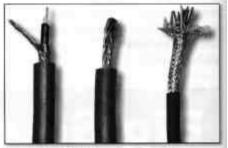
PHOTO 3: Shielded cables for audio.
