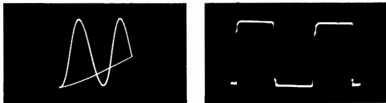
Fig. 1-34. These waveforms have the same peak-to-peak voltages, but their rms values are different.
