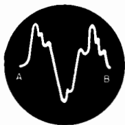
Fig. 1-40. Sweep magnifier action. Suitable for repetitive waveforms only.
