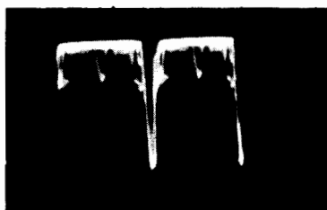
Fig. 4-5. Unsatisfactory sync separation.
