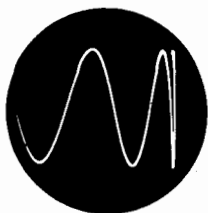
Fig. 1-27. Severe horizontal nonlinearity.
