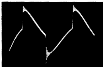
Fig. 3-26. Differentiation, ringing, and overshoot in a reproduced square wave.
