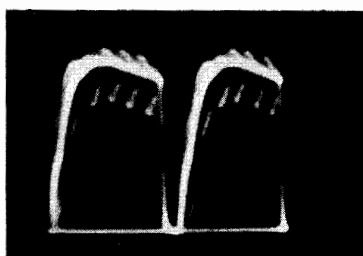
Fig. 5-9. Distorted waveform at point B when C4 is open.
