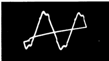
Fig. 2-13. Stray-field pattern, displayed when test leads of scope are left open.
