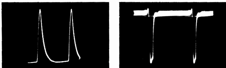
Fig. 4-15. Sync-separator outputs from two different receivers.
