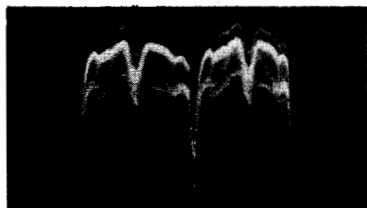
Fig. 3-6. Typical pattern obtained in an IF signal-tracing test.
