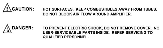
First, the tubes are hot... *really* hot. The 6AS7G tube in particular is specified to operate at up to 200° Celsius – that's 392° Fahrenheit. If you touch the tubes when the amplifier has been running for a while you will likely get burned.
