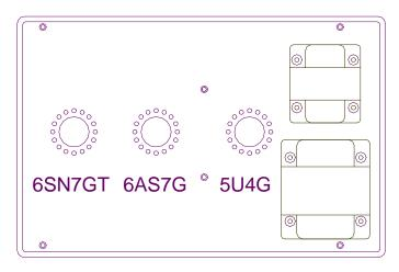
Make sure that the tubes are installed in the right locations. DOUBLE-CHECK! If you turn the amplifier on with the tubes in the wrong spots, you will likely ruin the tube, and may do damage to other amplifier components as well.
